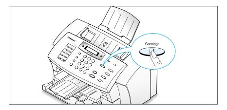
3. Lift the front panel by grabbing the panel along the top edge.
